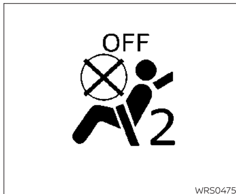
Front passenger air bag and status light
