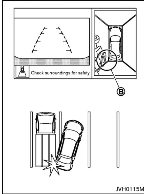
There may be a small distance visible between the vehicle and the object in the birdseye view on the display (B).
