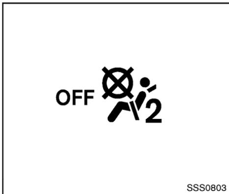
7. If the booster seat is installed in the front passenger seat, turn the ignition switch to the ON position. The front passenger air bag status light
