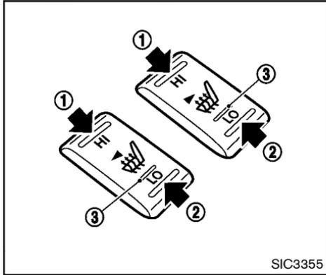
The heater is controlled by a thermostat, automatically turning the heater on and off. The indicator light will remain on as long as the switch is on.
