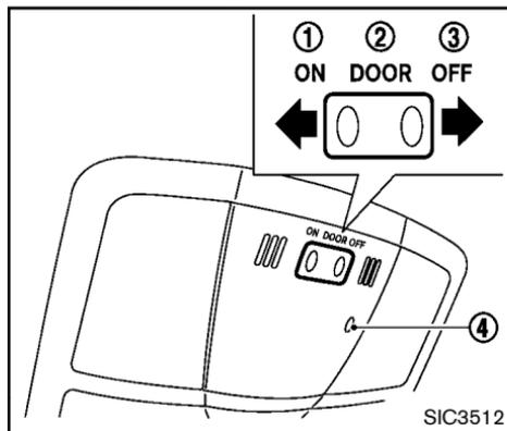
The map light control switch has three positions: ON ①, DOOR ② and OFF ③.
