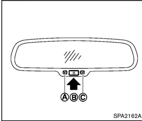
indicator light will turn off. Push the
