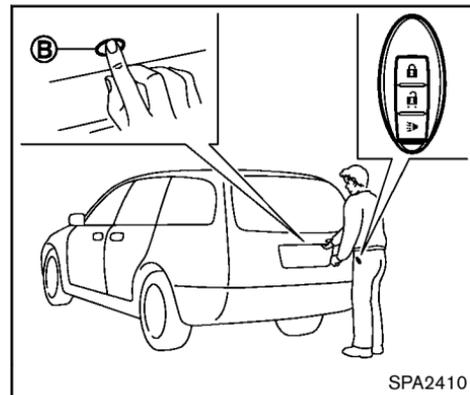
When you carry the Intelligent Key with you, you can lock or unlock all doors by pushing the door handle request switch (driver's or front passenger's) **(A)** or lift gate request switch **(B)** within the range of operation.
