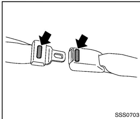
The center seat belt buckle and the tongue are identified by the CENTER mark. The center seat belt tongue can be fastened only into the center seat belt buckle.
