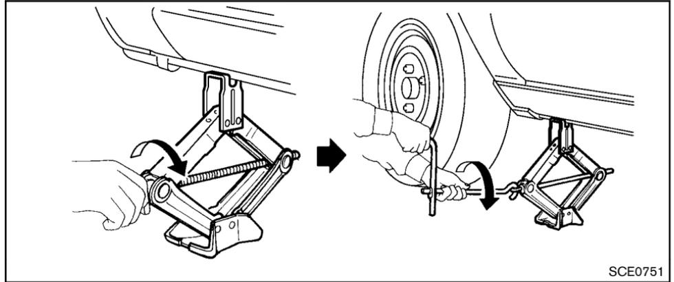
1. Place the jack directly under the jack-up point as illustrated so the top of the jack contacts the vehicle at the jack-up point. Align the jack head between the two notches in the front or the rear as shown. Also fit the groove of the jack head between the notches as shown.
