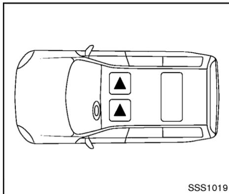
The illustration shows the seating positions equipped with head restraints. The head restraints are adjustable.
