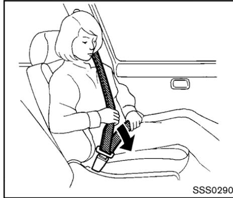
2. Slowly pull the seat belt out of the retractor and insert the tongue into the buckle until you hear and feel the latch engage.
