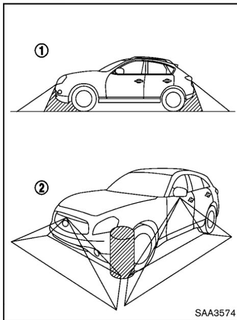
There are some areas where the system will not detect objects. When in the front or the rear view display, an object below the bumper or on the ground may not be detected ①. When in the bird's-eye view, a tall object near the seam of the camera detecting areas will not appear in the monitor ②.
