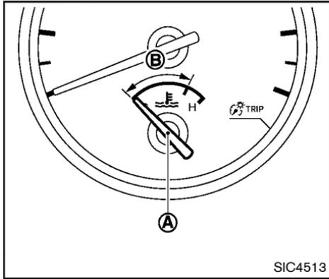
normal range, reduce vehicle speed to decrease temperature. If the gauge is over the normal range, stop the vehicle as soon as safely possible. If the engine is overheated, continued operation of the vehicle may seriously damage the engine. See “If your vehicle overheats” in the “6. In case of emergency” section for immediate action required.
