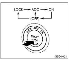
When the ignition switch is pushed without depressing the brake pedal, the ignition switch position will change as follows:
