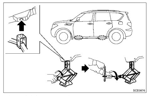
2. Loosen each wheel nut one or two turns by turning counterclockwise with the wheel nut wrench. Do not remove the wheel nuts until the tire is off the ground.
