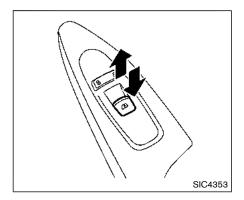
Passenger side power window switch The passenger side switch will open or close only the corresponding window. To open or close the window, push down or pull up the switch and hold it.
