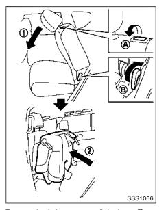
To enter the 3rd row seat, pull the lever (a) or (B) located on the 2nd row seat and fold the seatback forward (1) at an angle over the seat base. Then lift up the seat base and tip the 2nd row seat forward (2). This will release the back of the seat so it may be tipped forward.
