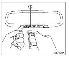
Using both hands, simultaneously press and hold the desired HomeLink<sup>®</sup> button and handheld transmitter button. DO NOT release until the HomeLink<sup>®</sup> indicator light (1) flashes slowly and then rapidly. When the indicator light flashes rapidly, both buttons may be released. (The rapid flashing indicates successful programming.)
