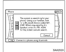
When a PIN code appears on the screen, operate the compatible Bluetooth<sup>®</sup> cellular phone to enter the PIN code.
