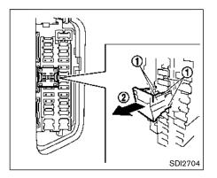
Extended storage fuse switch (if so equipped)
