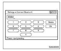
4. When a passkey appears on the screen, operate the compatible Bluetooth<sup>®</sup> audio device to enter the passkey. The pairing procedure of the audio device varies according to each audio device. See the Bluetooth<sup>®</sup> audio Owner's Manual for details.
