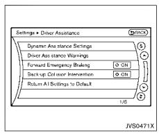
Highlight the "Back-up Collision Intervention" key, select ON (enabled) or OFF (disabled) and push the ENTER button (2).
