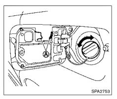
To remove the fuel-filler cap:
