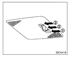
The cargo light switch has three positions: ON (1), center (2) and OFF (3).
