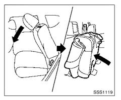
Push and hold the corresponding switch located on the instrument panel below the audio system. The seatback will fold down and tip forward. See "Entry to 3rd row seat" (P.1-5).
