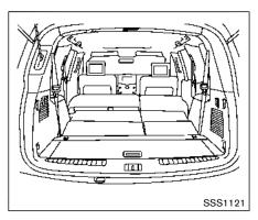
Power operation (if so equipped): Fold the 3rd row seat flat using the switches located in the cargo area. See "Power seat adjustment" (P.1-8).
