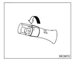
FOG LIGHT SWITCH (if so equipped) To turn the fog lights on, turn the headlight switch to the g position, then turn the switch to the  $\pm p$  position. To turn them off, turn the switch to the OFF position.
