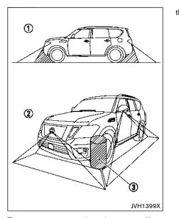
There are some areas where the system will not show objects and the system does not warn of moving objects. When in the front or the rear view display, an object below the bumper or on the ground may not be viewed ①. When in the bird's-eye view, a tall object near the seam ③ of the camera viewing areas will not appear in the monitor (2).
