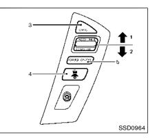
Vehicle-to-vehicle distance control mode switches
