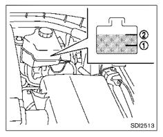
Check the fluid level in the reservoir. If the fluid is below the MIN line (1) or the brake warning light comes on, add Genuine NISSAN Super Heavy Duty Brake Fluid or equivalent **DOT 3** fluid up to the MAX line (2).
