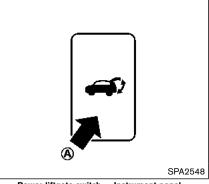
Power liftgate switch — Instrument panel
