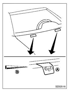
Be careful not to clog the washer nozzle  $(\underline{A})$ . This may cause improper windshield washer operation. If the nozzle is clogged, remove any objects with a needle or small pin  $(\underline{B})$ . Be careful not to damage the nozzle.
