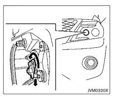
The high-beam headlight can be replaced from inside the engine compartment without removing the headlight assembly.
