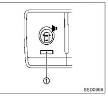
The warning systems switch is used to turn on and off the warning systems (Lane Departure Warning (LDW) and Blind Spot Warning (BSW) systems) that are activated using the settings menu on the center display.
