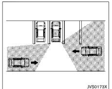
The radar sensors (A) detect an approaching vehicle from up to approximately 49 ft (15 m) away. The sonar sensors (B) detect stationary objects behind the vehicle up to approximately 4.9 ft (1.5 m). Refer to the illustration for approximate zone coverage areas ( $\hat{\mathbf{C}}$ ).
