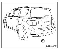
If dirt, rain or snow accumulates on the camera (1), RearView Monitor may not display objects clearly. Clean the camera by wiping it with a cloth dampened with a diluted mild cleaning agent and then wiping it with a dry cloth.
