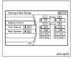
REAR DISPLAY settings (if so equipped) The rear display control screen will appear when the SETTING button is pushed, the "Rear Display" key is selected. (See "DVD Entertainment System" (P.4-92).)
