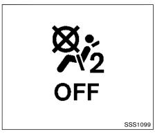
If the booster seat is installed in the front passenger seat, place the ignition switch in the ON position. The front passenger air bag status light images may or may not illuminate depending on the size of the child and the type of booster seat used. See "Front passenger air bag and status light" (P.1-60).
