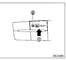
To defog/defrost the rear window glass and outside mirrors (if so equipped), start the engine and push the switch ① on. The indicator light ② will come on. Push the switch again to turn the defroster off.
