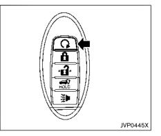
The remote engine start  $\mathbf{Q}$  button is on the Intelligent Key if the vehicle has remote engine start function. This function allows the engine to start from outside the vehicle.
