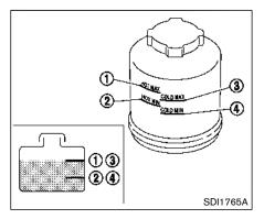
Check the fluid level in the reservoir.
