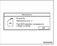
The Reminder will be automatically displayed when the specified distance has been driven and every time the ignition switch is pushed to the ACC or ON position. The reminder will not appear while driving.
