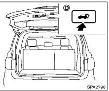
Power liftgate switch - Liftgate
