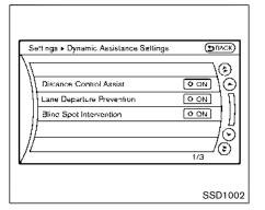
Highlight the "Distance Control Assist" key, select ON (enabled) or OFF (disabled) and push the ENTER button (2).
