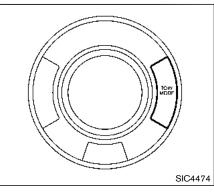
The TOW MODE should be used when pulling a heavy trailer or hauling a heavy load. Driving the vehicle in the TOW MODE with no trailer/load or light trailer/light load will not cause any damage. However, fuel economy may be reduced, and the transmission/engine driving characteristics may feel unusual.
