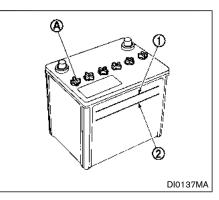
Check the fluid level in each cell (Remove the battery cover if it is necessary). It should be between the UPPER LEVEL ① and LOWER LEVEL ② lines.
