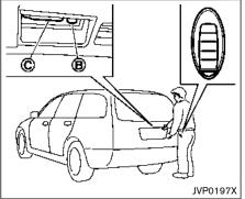
When you carry the Intelligent Key with you, you can lock or unlock all doors by pushing the door handle request switch (driver's or front passenger's) (a) or the liftgate request switch (B) within the range of operation.
