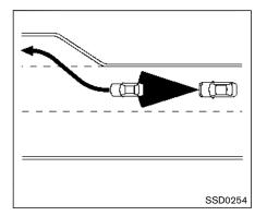
erates or decelerates your vehicle according to the speed of the vehicle ahead. Depress the accelerator to properly accelerate your vehicle when acceleration is required for a lane change. Depress the brake pedal when deceleration is required to maintain a safe distance to the vehicle ahead due to its sudden braking or if a vehicle cuts in. Always stay alert when using the ICC system.
