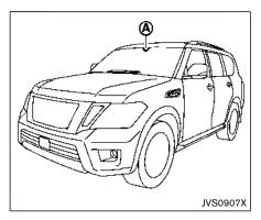
The LDW and LDP systems use a camera (A) installed behind the windshield to monitor the lane markers of your traveling lane.
