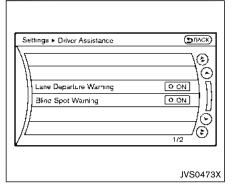
Highlight the "Blind Spot Warning" key, select ON (enabled) or OFF (disabled) and push the ENTER button (2).
