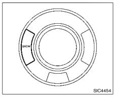
For driving or starting the vehicle on snowy roads or slippery areas, turn the SNOW mode on.
