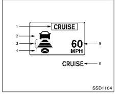
Vehicle-to-vehicle distance control mode display and indicators
