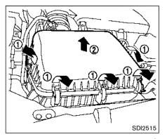
flame if the engine backfires. If it isn't there, and the engine backfires, you could be burned. Do not drive with the air cleaner removed, and be careful when working on the engine with the air cleaner removed.
