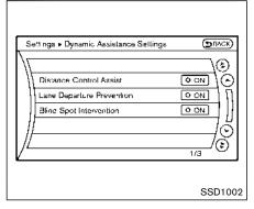
To set the LDP system to on or off, highlight the "Lane Departure Prevention" key, select ON or OFF and push the ENTER button
