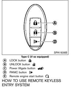
When you lock or unlock the doors or the liftgate, the hazard indicator will flash and the horn (or the outside chime) will sound as a confirmation. For details, see "Setting hazard indicator and horn mode" (P.3-17).
