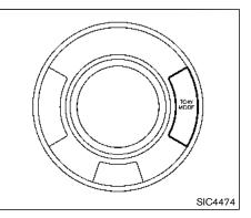
TOW MODE should be used when pulling a heavy trailer or hauling a heavy load. Driving the vehicle in TOW MODE with no trailer/load or light trailer/light load will not cause any damage. However, fuel economy may be reduced, and the transmission/engine driving characteristics may feel unusual.
