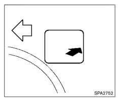
To open the fuel-filler door, unlock the fuel-filler door by using one of the following operations, then push the right side of the door.
