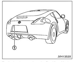
To display the rear view, the RearView Monitor system uses a camera located just above the vehicle's license plate (1).
