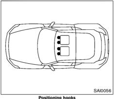
The illustration shows the location of floor mat positioning hooks.
