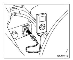
Open the console lid and connect the iPod® cable to the USB connector. If compatible, the battery of the iPod® is charged while the connection to the vehicle.
