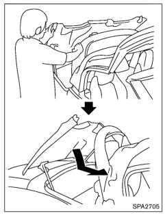
d. Pull down and slide the storage lid to close while holding the rear soft top from the right and left side of the vehicle.
