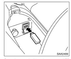
Open the console lid and connect a USB memory as illustrated. Then, push the DISC-AUX button repeatedly to switch to the USB memory mode.
