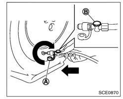
5. Remove the protective cap (a) of the hose and screw the hose securely onto the tire valve. Make sure that the pressure release valve (B) is securely tightened. Make sure that the air compressor switch is in the OFF (()) position, and then insert its power plug into the power outlet in the vehicle.
