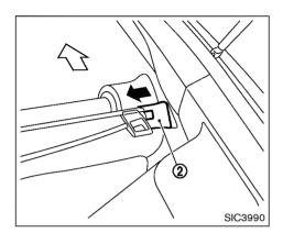
To remove the cargo cover unit, stow the cover and pull the holder (2) to the opposite side.
