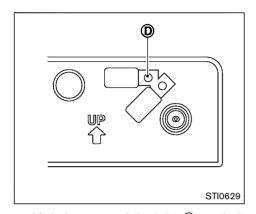
Mark the center of the hole (D) on both sides with a felt-tip pen. Remove the bracket from the bumper, and then open 0.9 to 1.0 inch (22 to 25 mm) diameter holes on the bumper using the marks (D) as a center.
