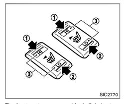
The front seats are warmed by built-in heaters. The switches located on the center console can be operated independently of each other.
