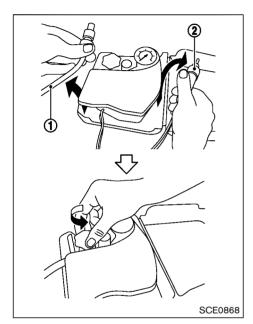
Take the hose (1) and the power plug (2) out of the air compressor. Remove the cap of the bottle holder from the air compressor.
