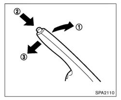
**To apply:** Pull the parking brake lever up (1). To release:
