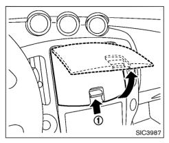
INSTRUMENT POCKET (except for navigation system equipped models) To open the lid, push the knob up (1).
