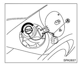
To remove the fuel-filler cap:
