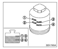
Check the fluid level in the reservoir.
