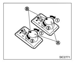
The climate controlled seat warms up or cools down the front seats by blowing warm or cool air from the surface of the seat. The switches located on the center console can be operated independently of each other.
