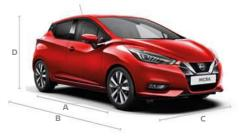
A: Wheelbase: 2,525 MM B: Overall length: 3,999 MM C: Overall width: 1,743 MM D: Overall height: 1,455 MM
